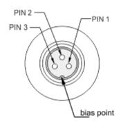
PIN 1 (RD)= 24VDC PIN 2 (BK)= 0V PIN 3 (GN)= Control
