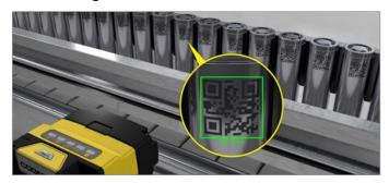
Increase traceability and operational efficiency by easily decoding direct-part marks.
